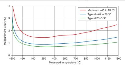
Figure 2. NI 9210 with Spring Terminal Thermocouple Type J and N Errors
