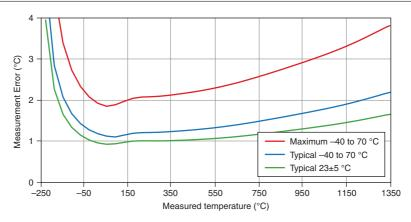
Figure 5. NI 9210 with Mini-TC Thermocouple Type T and E Errors
