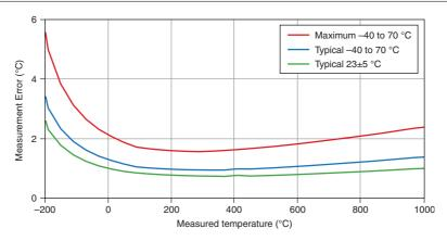
Figure 7. NI 9210 with Mini-TC Thermocouple Type B Errors
