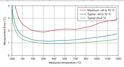
Figure 3. NI 9210 with Mini-TC Thermocouple Type K Errors
