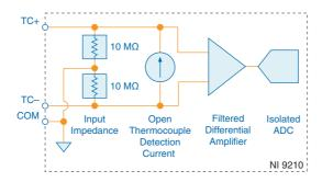
The channels of the NI 9210 share a common ground isolated from other modules in the system. Each channel passes through a filter and then a 24-bit analog-to-digital converter (ADC) samples the channel.
