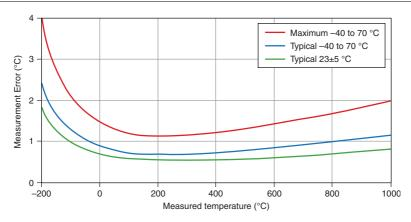
Figure 6. NI 9210 with Spring Terminal Thermocouple Type T and E Errors
